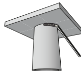
Pipe Fixed Horizontal Overhead Position PDH / 4F
